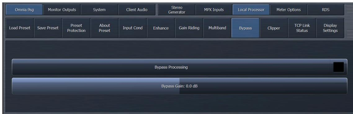
Enabling the “Bypass Processing” button bypasses all dynamics processing. The “Bypass Gain” control should be set so that the level of unprocessed (bypassed) audio matches the average level of process audio as closely as possible.
