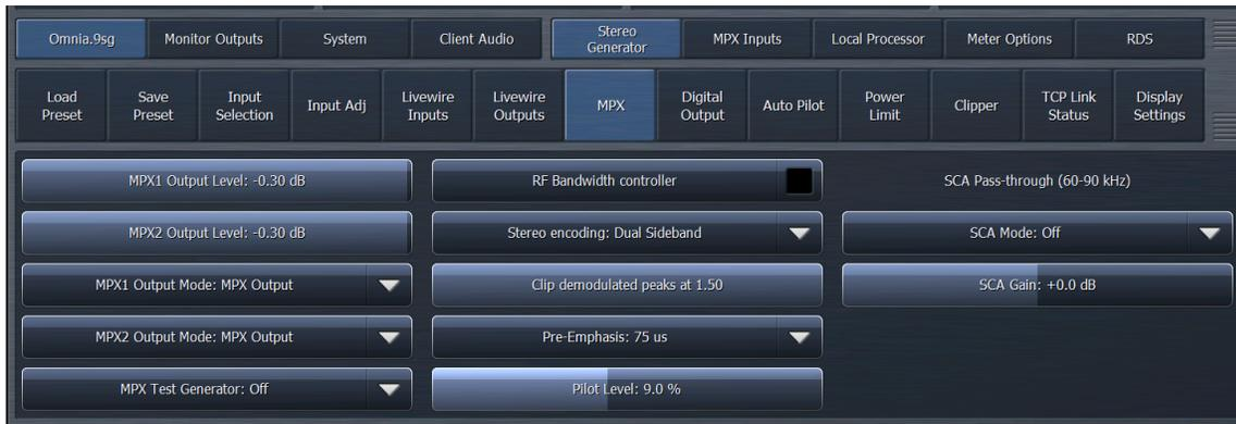
Adjustments that affect the normal composite outputs and the Omnia Direct composite over AES outputs are found here.
