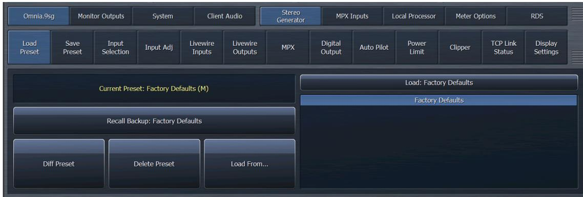
Once you have made changes to the various controls and settings, you will likely want to save those for easy and instant recall. These presets can then be recalled via the “Load Preset” menu. A list of available presets appears on the right side of the screen. Those displayed in white are factory presets. Those displayed in yellow are user presets.
