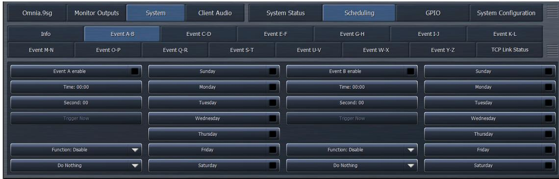
The controls in the Scheduling menu allow you to program up to twenty-six day- and time-driven events including changing the local input mode (on units so equipped), triggering internal playback, and presets in the stereo generator, local processor, and monitor outputs. Any custom task scripts can also be executed by the scheduler.
