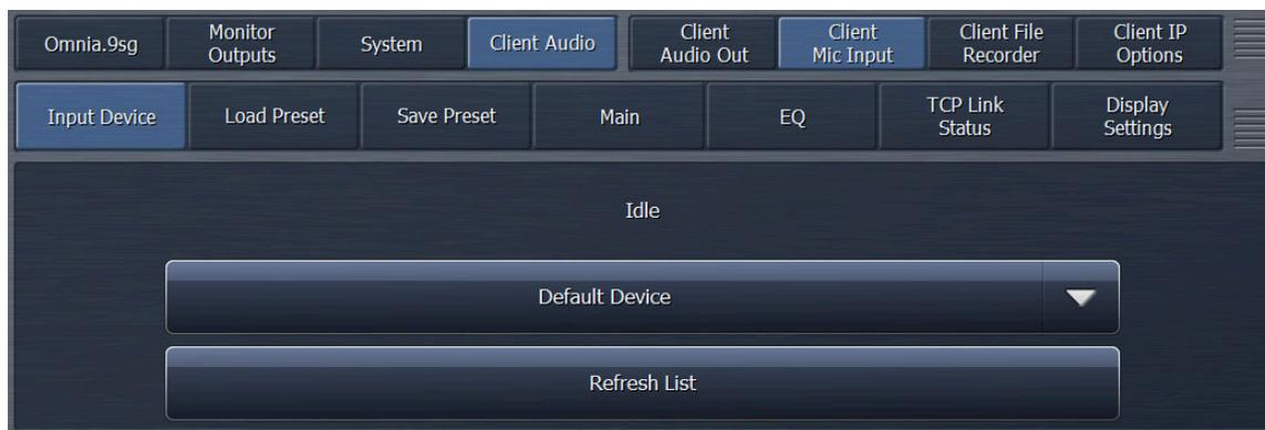
The Client Microphone Input Menu allows you to pick which microphone you’d like to use, a parametric equalizer to create custom EQ curves for individual mics, and the ability to save and recall custom mic presets.
