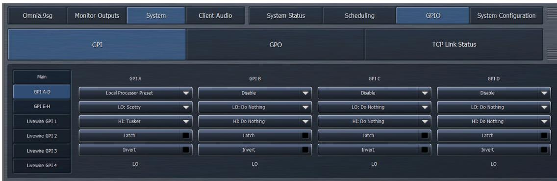
GPI functionality is enabled or disabled in the “Main” tab. Please note that GPI must be disabled in order to make any GPI configuration changes.
