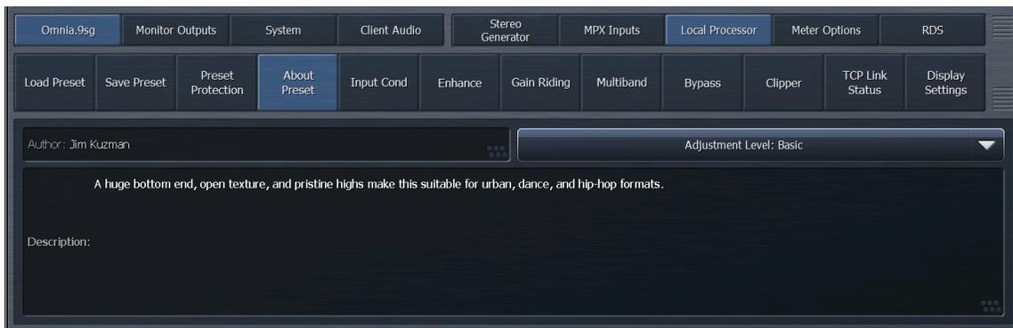
The “About Preset” menu contains information about the current preset including its current adjustment level (Basic, Intermediate, Expert), its author, and a description of its characteristics.
