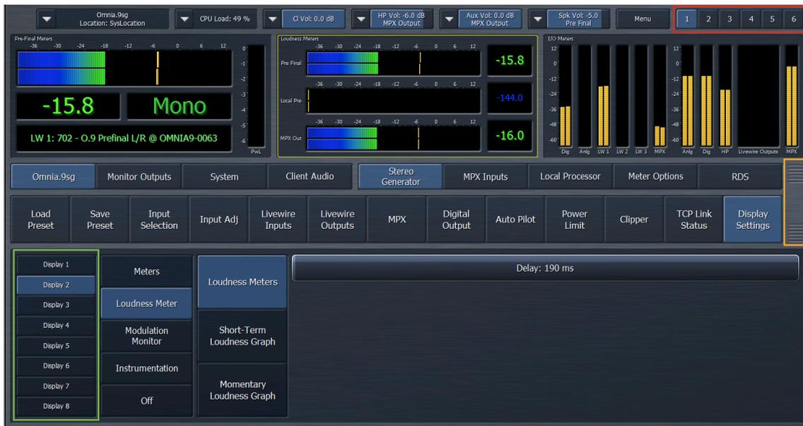
A row of six “Display Preset” buttons is located at the top right corner of the NfRemote display, outlined here in red. Each display preset can show up to eight display windows, outlined here in green. The number of simultaneous displays used in each preset will depend primarily upon monitor size as adding displays reduces the size of each individual window and will, on smaller monitors, quickly make them less readable and useful.
