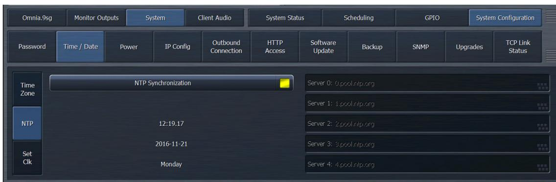
Again, this one should be fairly self explanatory. This menu allows setting the time zone, enabling time sync via NTP servers, or setting the clock manually. We recommend that you use NTP if at all possible—particularly if you intend to broadcast time via RBDS.
