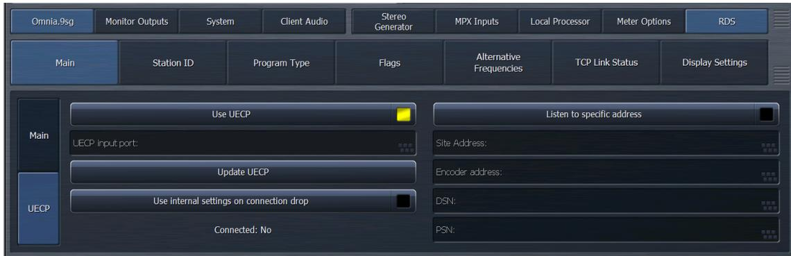
UECP (Universal Encoder Communications Protocol) is a standardized protocol for communicating with RDS encoders and provides the ability to address all encoders, specific groups of encoders, or individual encoders. This is particularly useful in non-U.S. applications where the use of RDS is more highly developed and embraced and where identical content is broadcast from multiple geographically-diverse transmitter sites.
