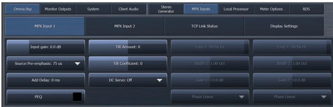
Omnia.9sg offers two rear panel composite (MPX) inputs which can be used to feed the output of an external RDS generator, the composite output of another processor, or the composite output of a tuner or frequency-agile modulation monitor.
