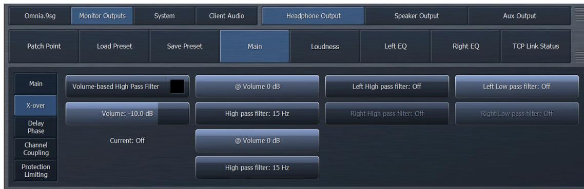
The “Main Menu” contains controls that allow high-pass and low-pass filter frequencies to be set and also permit different high pass filtering depending upon the setting of the “Volume” control. This can compensate for systems that have an uneven frequency boost applied to make them sound better at low volumes which does not scale appropriately with increased volume.
