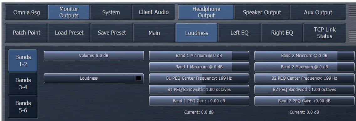
The audio monitoring tools in 9sg also include a loudness curve adjustment. These controls (much like the “Volume-Based High Pass Filter” mentioned earlier) can compensate for monitoring systems with an uneven frequency response that varies based on the volume. There are 6 bands of control available (displayed in groups of 2) and all function identically.
