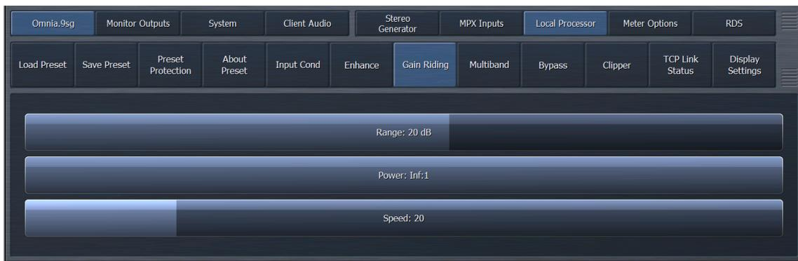
The behavior of the wideband AGC’s (Input AGC and Wideband AGC) is determined by the settings of the controls in this menu.
