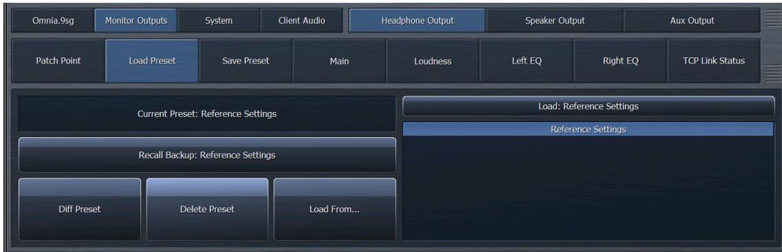
Because Omnia.9sg (along with the “Client Audio” feature built into NfRemote) provides all of the tools – minus a calibrated microphone – to perform speaker/room calibrations for each Monitor Output, it also provides a means by which to store those calibrations for later recall in the form of presets.
