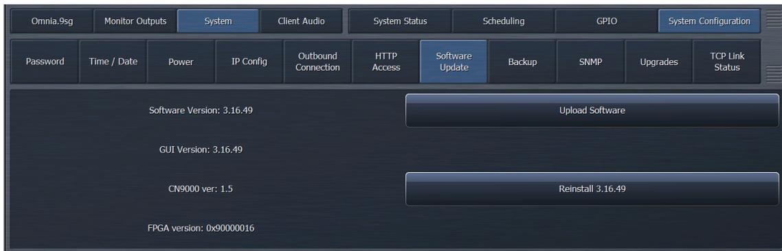
The “Software Update” menu displays the current 9sg software (and NfRemote client) version as well as the versions associated with several internal 9sg components.
