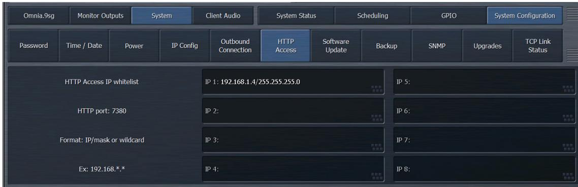
In addition to access via NfRemote, the 9sg has an extensive http remote control interface built in. It is not necessary to configure these settings if you do not plan to use the http interface. This menu **ONLY** controls access via the remote http interface and does **NOT** restrict access via NfRemote.
