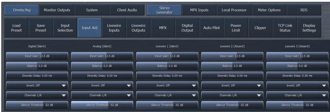
All controls affecting the signal at the input of the clipper are located here.
