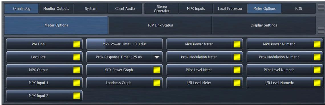
Exactly which meters appear in the Loudness Meter, Modulation Meter, and Modulation Numeric display windows is determined by enabling or disabling various options in this menu. If you do not see a meter you expect to see in any of the graphs or meters, check this menu to ensure the one you are looking for has been enabled.
