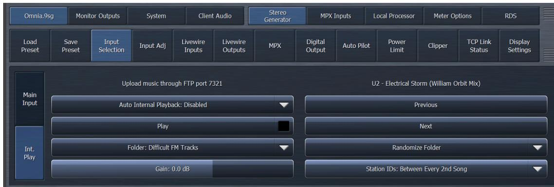
Omnia.9sg also offers an internal playback feature designed to keep you on the air in the event the primary and secondary sources become unavailable, perhaps due to the failure of an STL or a play-out system at the studio.
