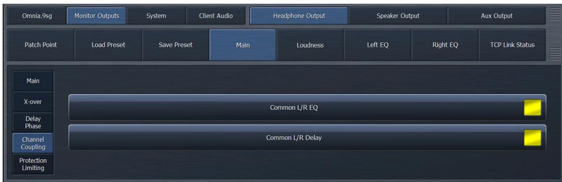
In some installations, the left and right speakers are in similar locations within the room and relative to the monitoring point. In these situations, EQ and Delay settings can be applied to both channels by enabling the “Common L/R EQ” and “Common L/R Delay” controls.
