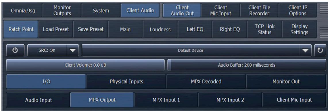
To enable client audio output, click the “power button” icon in this menu. A selectable Sample Rate Converter (SRC) ensures that the audio remains stable, though when enabled this feature consumes additional CPU resources.
