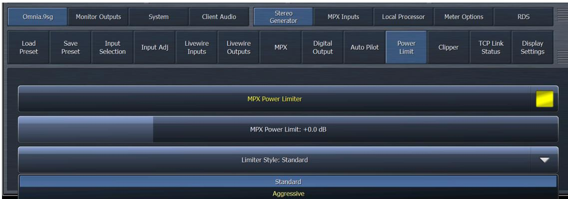
ITU-R BS.412 standards require the average MPX power to be limited to a particular standard and measured with a rolling 60-second integration time. It is assumed that whatever processor is feeding Omnia.9sg will employ processing presets optimized for power limiting.
