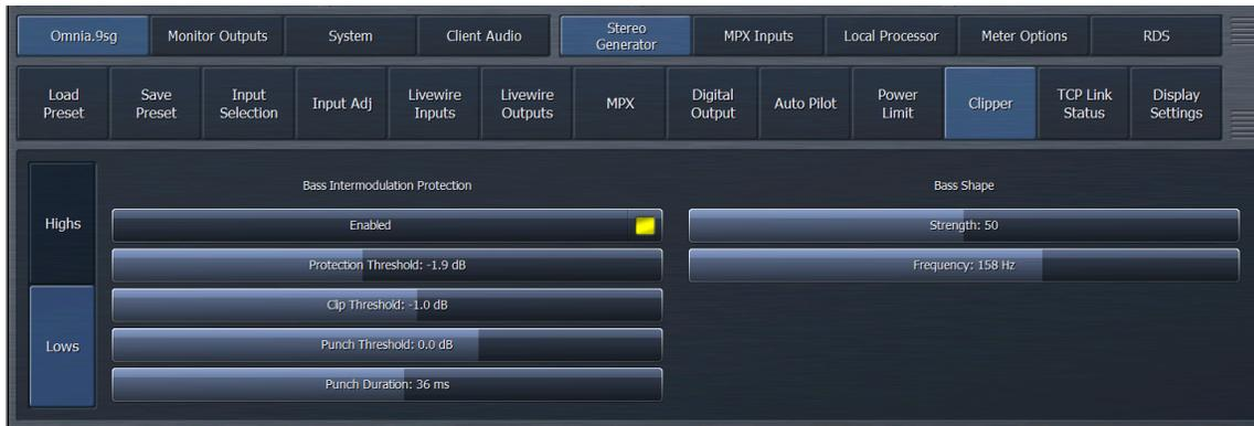
These controls affect the texture and feel of the bass clipper and are sub-divided into two groups: “Bass Intermodulation Protection” and “Bass Shape”
