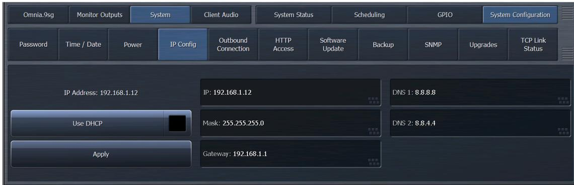
This menu allows configuration of the unit’s IP address, subnet mask, gateway, and DNS servers. It also allows you to select configuration via DHCP. The currently assigned IP address is one of the first items displayed in this menu.
