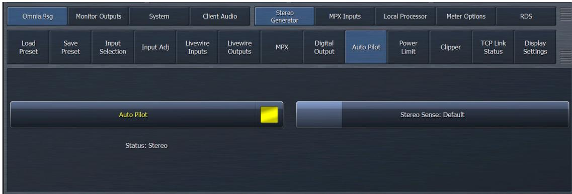
As explained in detail earlier in the manual, Auto Pilot allows the stereo pilot to be turned off when source material is mono and seamlessly re-enabled when the source is stereo, providing significant improvements to noise levels and multipath distortion.
